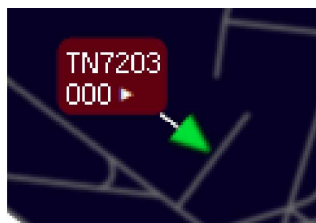
Plate 30: IFF – An aircraft after pressing the IDENT switch on the transponder.
